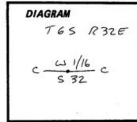
Description of corner evidence found: 3 1/4" BLM BRASS CAP MKO:  $c \frac{W 1/16}{S 32} c$  set on 2 1/2" iron post, in A mound of stone, From which:
