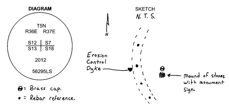
MONUMENT (S) AND ACCESSORIES SET (Procedures and Description) I set a 2 3/8" brass cap on a 1 1/2"x30" galvanized iron pipe with a brass cap stamped as shown in the diagram above 28" in the ground to bedrock at the proportionate point.
