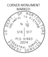
Painted a 6" red band around each bearing tree, and also painted blazes red and attached USFS 54-3 and 54-9 signs. Distances measured with a steel tape to a 60d nail driven in the right-side-center above the root crown, with a  $1\frac{1}{2}$ " aluminum washer stamped PLS 91693. Bearings measured with a handheld compass with  $14^\circ$  east declination. Set aluminum posts, 3 ft. north and 5 ft. east with USFS 54-9 and 54-2 signs attached. Monument lies 5 ft.west of a north-south fence-line.
