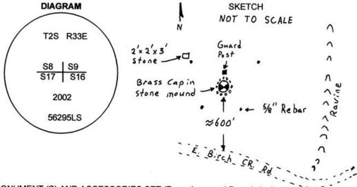
MONUMENT (S) AND ACCESSORIES SET (Procedures and Description) Set a 11/2" x 30" galvanized iron pipe with a 2 1/4" brass cap stamped as shown in the diagram 15" in the ground at the position of the original stone. Burried the stone along the east side of the monument. Attached a county monument sign to a 5' steel guard post.
