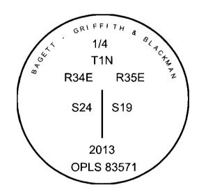
I used a steel tape and magnetic compass in the recovery of the bearing trees and establishment of new tree. I used 16° East magnetic declination and the bearings and distances are to the center of root crown on old bearing trees. Distance is to a 60d spike in the right hand side of the new trees. Bearing is to a brass washer marked OPLS 83571 in the lower BT blaze.
