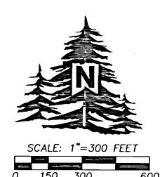
"BASIS OF BEARINGS." BEARINGS ARE TRUE BASED ON A GEODETIC GPS OBSERVATION TAKEN AT THE NORTH 1/4 CORNER OF SECTION 20. ROTATE COUNTER-CLOCKWISE 1.26615206, AND SCALE 0.999872279 (C.F.) TO OBTAIN GRID BEARINGS AND DISTANCES.
