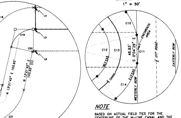
BASED ON ACTUAL FIELD TIES FOR THE CENTERLINE OF THE M-LINE CANAL AND THE FOUND SECTION LINE MONUMENTS IT APPEARS THAT THE EASTERLY EASEMENT LINE OF THE CANAL FALLS WITHIN THE RIGHT OF WAY OF OTT ROAD AS SHOWN IN THE DETAIL.
