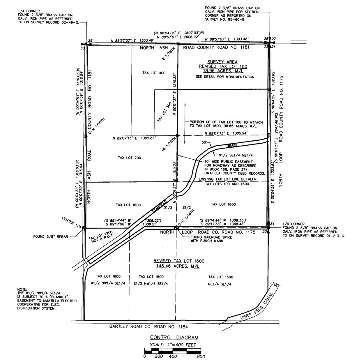
NOTE: SURVEY DIMENSIONS SHOWN ON THE CONTROL DIAGRAM ARE BETWEEN CORNERS ON SECTION OR SECTION BREAKDOWN LINES.
