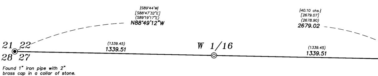
Found 1" iron pipe with 2" brass cap in a collar of stone 5/8" iron pin with plastic cap marked LS645 bears N30°E, 0.10 feet.
