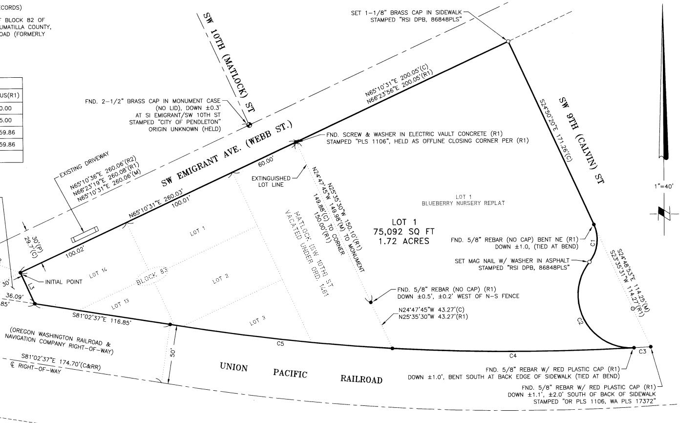
1. BASIS OF BEARING IS GRID, OREGON STATE PLANE, NAD\_83(2011), NORTH ZONE BASED ON GPS OBSERVATIONS. DISTANCES SHOWN HEREON ARE 'GROUND' SCALED FROM GRID USING A COMBINED FACTOR OF 0.99988500 FROM LATITUDE: 45'40'02.0"N LONGITUDE: 118'47'39.8"W.
